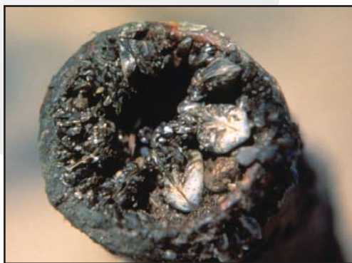
Zebra Mussels Clogging a Pipe Photo Courtesy of Michigan Sea Grant ( www.miseagrant.umich.edu )
